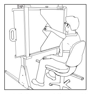
*Figure 1.* Adjustable aperture apparatus. Participants sat on a swivel chair and reached through the aperture for a target. Between trials, participants turned away from the aperture while an experimenter adjusted the size of the aperture by pulling the handle.
