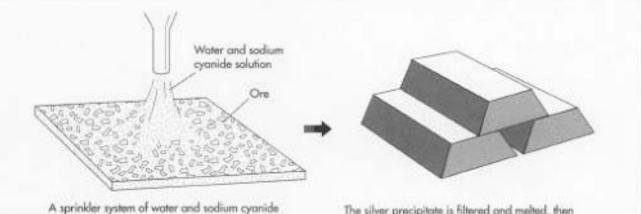
A sprinkler system of water and sodium cyanide is applied to the ore. Zinc dust is then added to remove the precious metal from the solution. The silver precipitate is filtered and melted, then formed into bullion bars.
