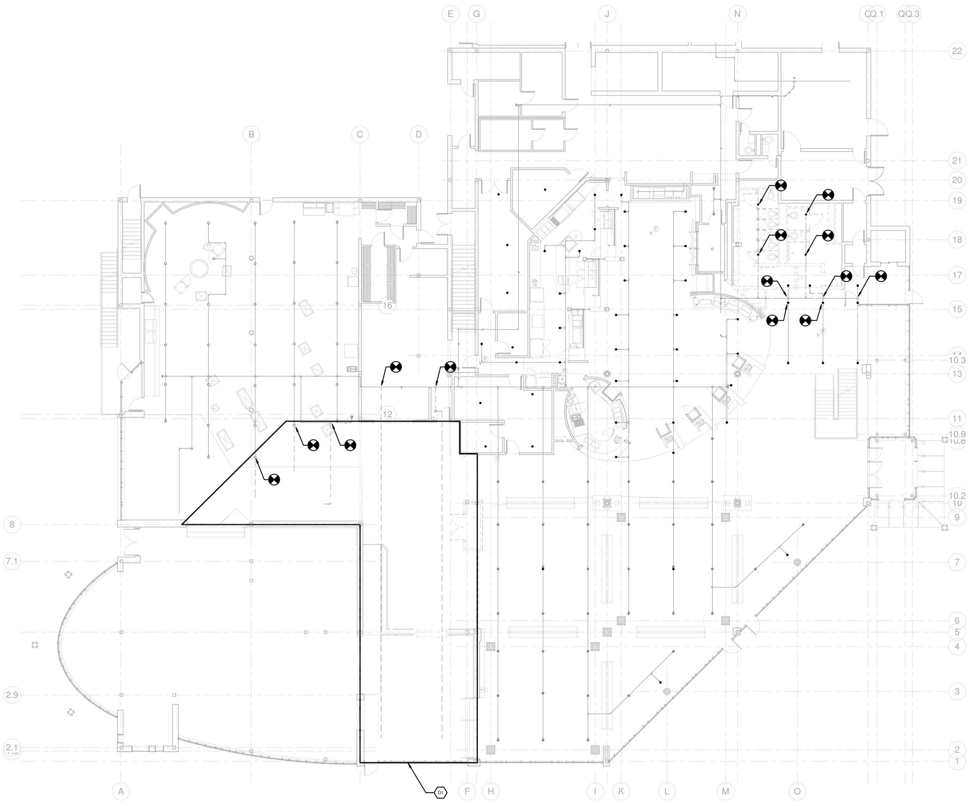
**1** PHASE 2 INTERIOR - FIRE PROTECTION DEMOLITIONS - FIRST FLOOR
