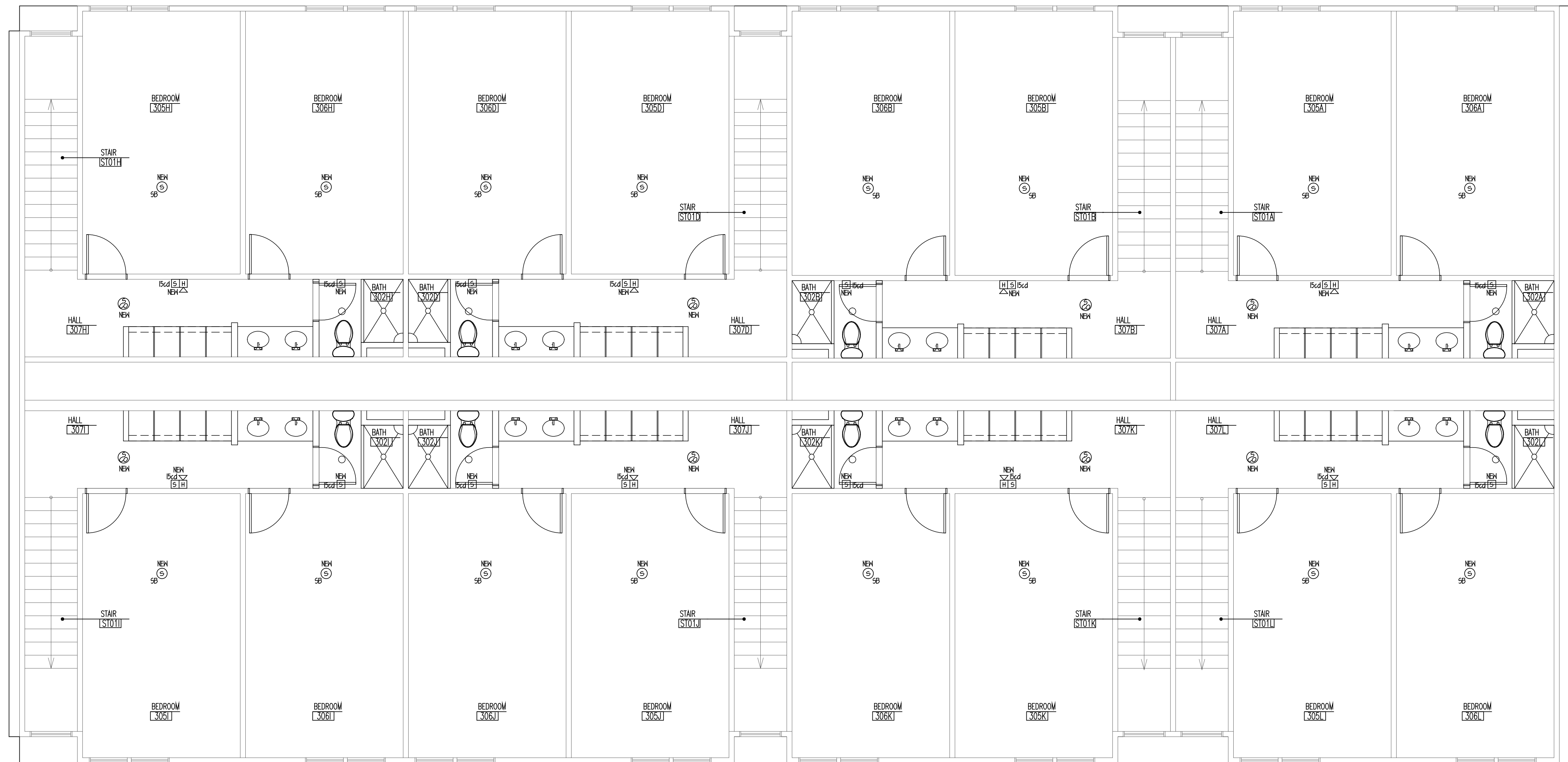
THIRD FLOOR FIRE ALARM PLAN SCALE: 1/4"=1'-0"
